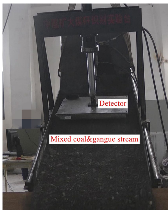
Figure 9. Top coal caving simulation test.
