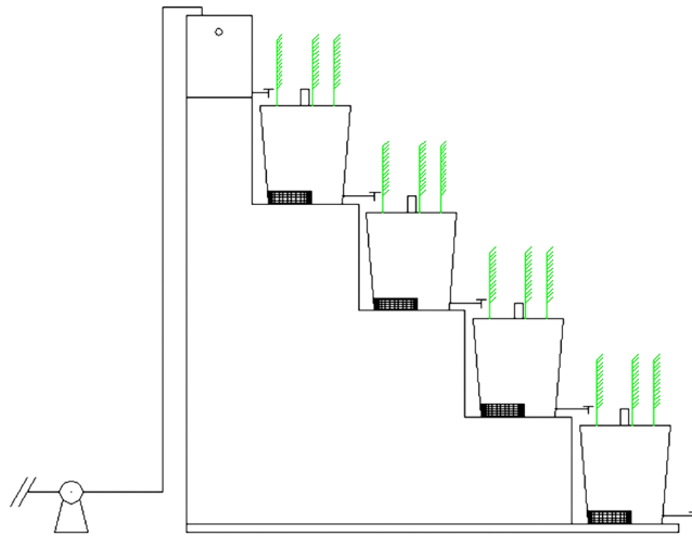
Figure 1. Schematic diagram of dewatered alum sludge-based sequencing batch constructed wetland system.
