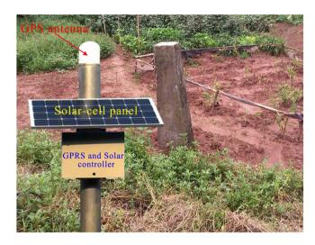
Figure 5. GPS reference and measuring points on Wangmiao landslide.
