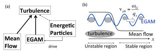
**Figure 1.** (a) Model on relationship between turbulence, mean flow, EGAM and EPs. (b) Model geometry of the inhomogeneous turbulence with the mean flow.
