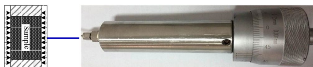
Figure 6. Volumetric strain measurement device.
