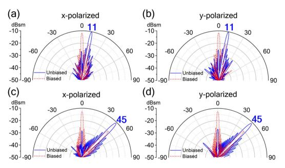
**Figure 6.** Metasurface designs for different single beam switching. (**a**,**b**) 2D Far-field patterns of the singlebeam switching metasurfaces given in polar coordinates indicating beam switch between 0° and 11°, (**c**,**d**) or beam switch between 0° and 45° under normal incidence of (**a**,**c**) *x*- and (**b**,**d**) *y*-polarization at 1.0 THz. (The blue number indicates the direction angle of the switched beam).
