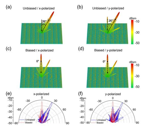
**Figure 4.** Simulated far-field scattering patterns. 3D far-field scattering patterns in the (**a**,**b**) unbiased and (**b**,**d**) biased state, (**e**,**f**) 2D Far-field patterns given in polar coordinates for two voltage states of the single-beam switching metasurface under normal incidence of (**a**,**c**,**e**) *x*- and (**b**,**d**,**f**) *y*-polarization at 1.0 THz.
