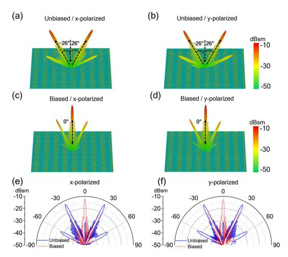
**Figure 7.** Metasurface designs for dual reflection beam switching. 3D Far-field scattering patterns in the (**a**,**b**) unbiased (main lobe at direction angles of  $\pm 26^{\circ}$ ) and (**c**,**d**) biased (main lobe at 0° direction angles) state, as well as (**e**,**f**) 2D Far-field patterns given in polar coordinates for two voltage states of the dual beam switching metasurface under normal incidence of (**a**,**c**,**e**) *x*- and (**b**,**d**,**f**) *y*-polarization at 1.0 THz.
