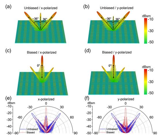
**Figure 8.** Metasurface designs for dual reflection beam switching. 3D Far-field scattering patterns in the (**a**,**b**) unbiased (main lobe at direction angles of  $\pm 36^{\circ}$ ) and (**c**,**d**) biased (main lobe at 0° direction angles) state, as well as (**e**,**f**) 2D Far-field patterns given in polar coordinates for two voltage states of the dual beam switching metasurface under normal incidence of (**a**,**c**,**e**) *x*- and (**b**,**d**,**f**) *y*-polarization at 1.0 THz.
