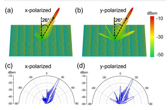
**Figure 2.** Simulated far-field scattering patterns. (**a**,**b**) 3D far-field scattering patterns, and (**c**,**d**) 2D far-field scattering patterns in polar coordinates for the anomalous reflection metasurface under normal incidence of (**a**,**c**) x-, and (**b**,**d**) y-polarization at 1.0 THz.
