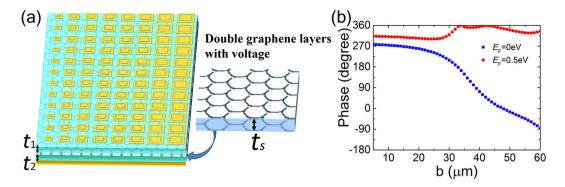
**Figure 3.** Single-beam switching metasurface. (a) Schematics of the metasurface, with right part representing the gated structure consisting of double graphene layers sandwiched with a thin silicon dioxide insulating film. (b) The reflection phase of the unit cells as functions of the dimension *b* at 1.0 THz for  $E_F = 0$  eV (blue square) and  $E_F = 0.5$  eV (red filed circle), respectively.
