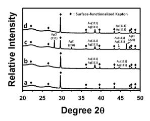
**Figure 4.** X-ray diffraction (XRD) analyses of (**a**) the starting Kapton<sup>®</sup> substrate (functionalized with the SWCNT-selector complexes), (**b**) the inkjet-printed Kapton<sup>®</sup>-Ag structure after the annealing but before the Ag-to-Au conversion, (**c**) the Kapton<sup>®</sup>-IDE structure after the Ag-to-Au conversion but before the selective removal of the AgCl, and (**d**) The Kapton<sup>®</sup>-IDE structure after the selective removal of the AgCl.
