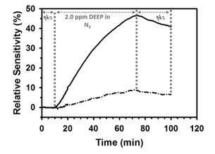
**Figure 5.** Typical sensing behavior of the proof-of-concept SWCNT-based sensors with dense Ag IDEs (dashdot line) and with porous Au IDEs (solid line) upon exposure to 2.0 ppm DEEP vapour.
