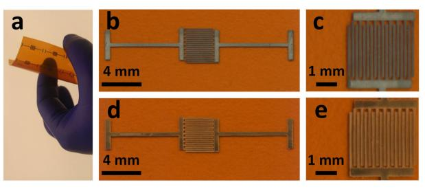
**Figure 1.** Scanned images of the inkjet-printed sensors before (**a**,**b** and **c**) and after (**d** and **e**) the conversion of the Ag IDEs into their Au counterparts.
