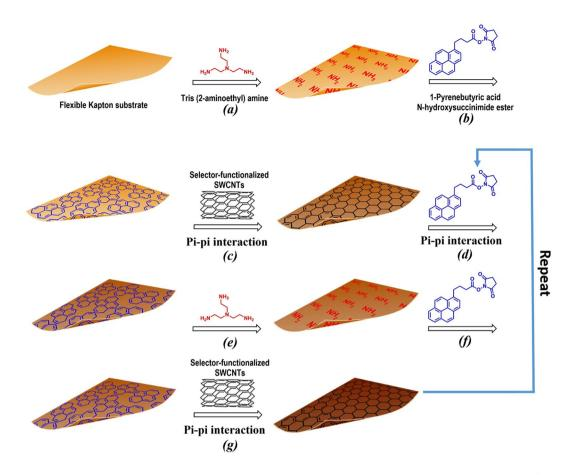
**Figure 6.** Layer-by-layer deposition of the SWCNTs and the chemoselective molecules on a flexible Kapton<sup>®</sup> substrate.
