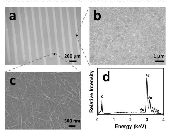
**Figure 2.** Scanning electron microscopy (SEM) and energy dispersive X-ray spectroscopy (EDX) analyses of a sensor before the Ag-to-Au conversion. (**a**) SEM image of the sensor; (**b**) SEM image focusing on an IDE finger of the sensor; (**c**) SEM image focusing on the SWCNT-selector complexes between two adjacent IDE fingers; (**d**) EDX pattern of the specimen shown in (**b**).
