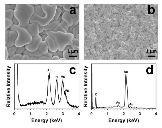
**Figure 3.** SEM images and EDX patterns of the IDEs of an SWCNT-based sensor at different stages after the Ag-to-Au conversion. (**a**) SEM image of the IDEs after the Ag-to-Au conversion but before the removal of the side product AgCl; (**b**) SEM image of the IDEs after the Ag-to-Au conversion and the removal of the side product AgCl; (**c**) and (**d**) EDX patterns of the specimens shown in (**a**) and (**b**), respectively.
