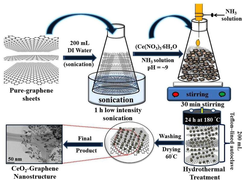
Figure 12. Schematic representation for the synthesis steps of the CeO 2 -Graphene nanostructures.
