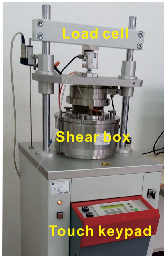
Figure 1. The commercially available soil mechanics ring-shear apparatus used in the study.
