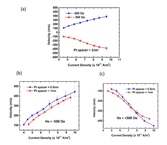
**Figure 4.** (a) DW velocity versus current density in the presence of a constant in-plane magnetic field in +x and -x-directions for 1-nm-thick Pt spacer; plot symmetry across x-axis reveals low DMI strength. DW velocity for Pt spacer with thicknesses 0.5 nm and 1 nm when a magnetic field was applied along (b) -x-direction, and (c) +x-direction. Comparison indicates increasing Pt spacer thickness reduces velocity.
