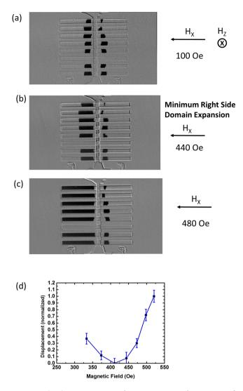
**Figure 2.** (**a**–**c**) Kerr imaging to show DW creep in the presence of out-of-plane and in-plane magnetic field. The in-plane field opposes DMI field for DW propagating towards right and minimum displacement occurs at field equal to DMI field. Here  $H_{DMI} = 440$  Oe. (**d**) Domain wall displacement as a function of in-plane magnetic field.
