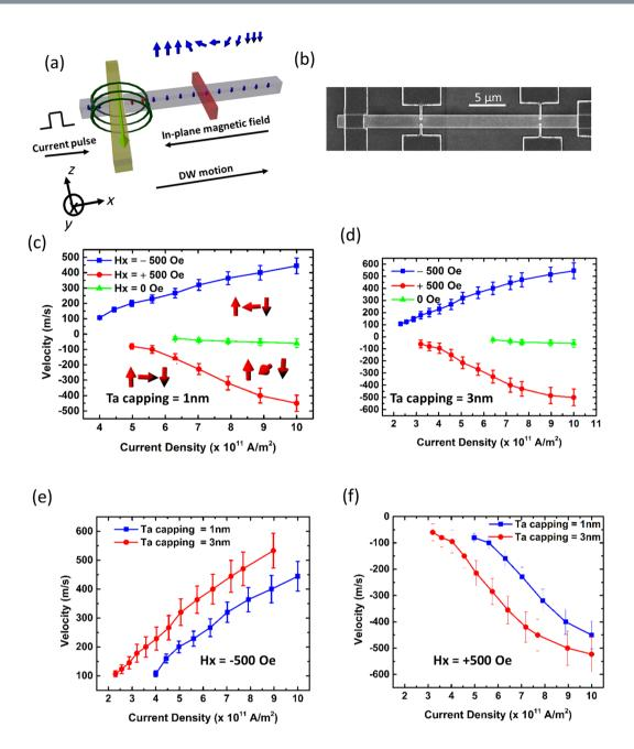
**Figure 1.** (a) Schematic depicting the setup for domain wall (DW) injection and driving measurement. (b) SEM image of the wire with non-magnetic Hall probes for DW detection. DW velocity versus current density under a constant in-plane magnetic field along + x and -x-directions for Ta capping with thickness (c) 1 nm, and (d) 3 nm. Comparison of DW velocity for Ta capping thicknesses 1 nm and 3 nm; magnetic field was applied along the (e) -x-direction, and (f) + x-direction.
