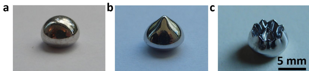
Figure 7. Instability pattern morphology formed by undercooled liquid Co under different magnetic fields, (a) without magnetic field, (b) 1 T magnetic field and a field gradient 15 T/m and (c) 4 T magnetic field and a field gradient 60 T/m.
