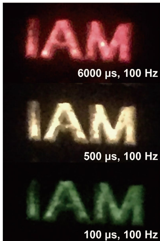
Figure 4. The photograph of tunable emission color of \text{NaYF}_4:\text{Er/Tm}@NaYF_4 nanoparticles under pulsed laser excitation for anti-counterfeiting. The size of one character is 3\text{ mm} \times 3\text{ mm} .
