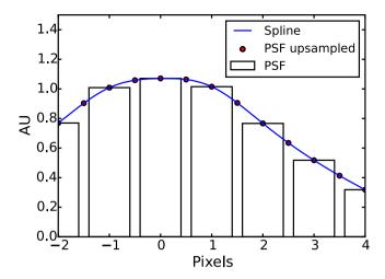
**Figure 1.** 1D Spline example. Each cubic spline interval (the blue line) is determined such that itself and its first derivative are continuous across the red points which are the interval boundaries. The red points are calculated by up-sampling the measured PSF (grey bars) by a factor of two using 3<sup>rd</sup> order spline interpolation.
