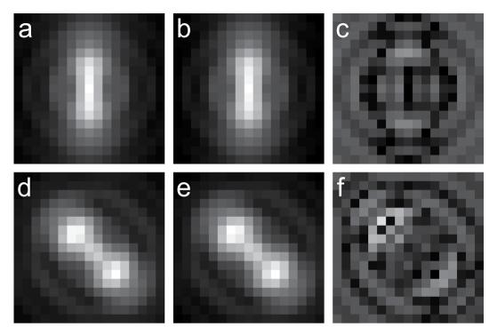
**Figure 2.** Analytical PSFs and their spline representations for the astigmatic PSF and saddle-point PSF. (a) Astigmatic PSF at z = -420 nm. (b) Cubic spline representation of (a). (c) Difference between (a) and (b) multiplied by 100. (d) Saddle-point PSF at z = -420 nm. (e) Cubic spline representation of (d). (f) Difference between (d) and (e) multiplied by 100.
