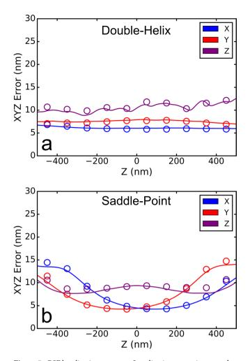
**Figure 5.** PSF localization accuracy. Localization errors in x, y and z are plotted as a function of z. (a) Double helix PSF. (b) Saddle-point PSF. The solid lines are the Cramer-Rao theoretical bounds calculated following ref. 8.
