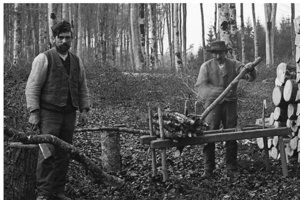
Fig. 3 Photograph illustrating the production of standardized bundles of small (<7 cm in diameter) woody parts of stem, i.e. tree top, and branches. Photo ‘Wellenmacher an der Arbeit’ (Preparation of bundles) in a Bernese forest by Herrmann Knuchel, 17.11.1916 from the collection of the Swiss Federal Research Institute WSL, reference no. EAF_00831_G_neg.
