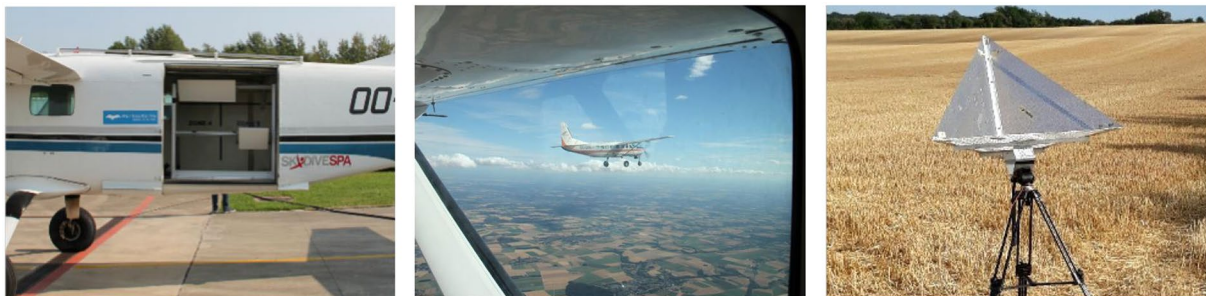
Fig. 2 MetaSensing B.V.'s SAR system on-board one of the two CESNA Gran Caravan airplanes (left), a picture of one airplane taken from the other while flying in the across-track (XTI) configuration (middle), and a corner reflector in the field (right).
