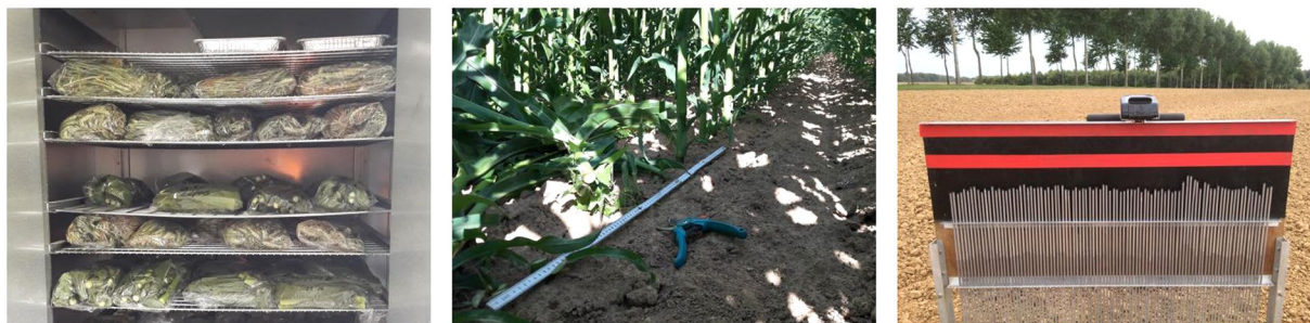
Fig. 7 Oven drying of the plant subsamples (left), crop cutting along a 1 m row (middle) and pin profilometer (right).
