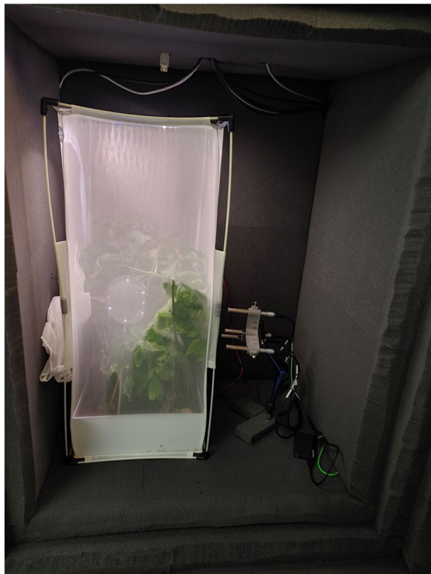
Fig. 3 View of the recording setup for the InsectSound1000 dataset inside the anechoic box. An illuminated insect-rearing cage containing a square plant pot with two tomato plants, a low-budget microphone array and one selected species of insect was placed inside the box to the left. Next to it is the high-quality microphone array, which consists of 4 low-noise measurement microphones.
