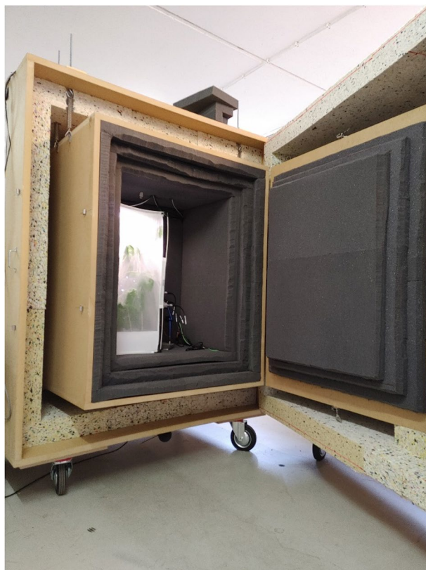
Fig. 1 Recording setup for the InsectSound1000 dataset. Double-wall anechoic box containing a microphone array and insect rearing cage.
