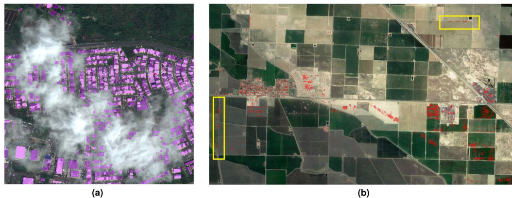
Fig. 5 Example of unfavorable structure extraction outcomes due to poor image quality or overly complex patterns that are not able to be removed during automatic QA/QC. (a) Raw structure extraction results colored in purple. Note the omissions due to the clouds. (recreated from 4 ). (b) Additional false positives that require manual QA/QC. The false positives in the yellow boxes are particular difficult to filter out by VVM.
