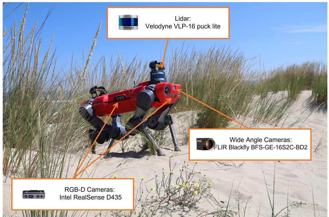
Fig. 1 The robot ANYmal C in habitat 2120 with highlighted the sensors used for acquiring data. These sensors are one Velodyne VLP-16 puck lite, two FLIR Blackfly BFS-GE-16S2C-BD2 wide angle cameras, and four Intel RealSense D435 RGB-D cameras.
