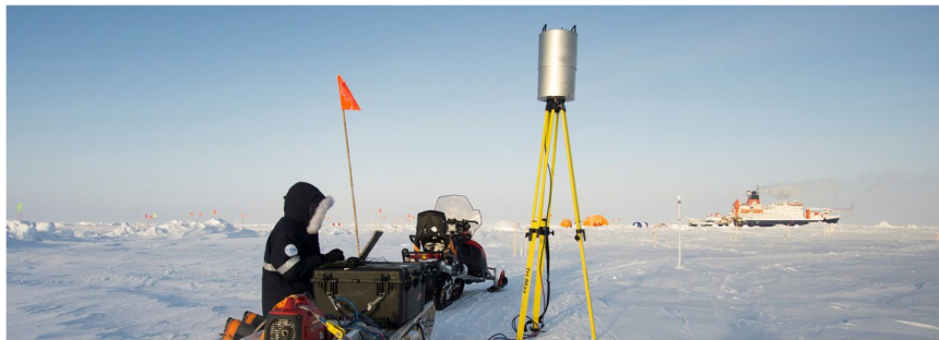
Fig. 1 Photo showing data acquisition of a typical scan position. The Riegl VZ1000 terrestrial laser scanner is inside the custom heater case (metal cylinder) on top of the tripod. The researcher controls the scanner from the laptop via WiFi. To the right of the tripod is a Riegl 10 cm cylinder reflector mounted on a post frozen into the ice. The Polarstern can be seen in the background along with other installations of the ice camp including Balloon Town 3 (orange tents) and Ocean City 4 (blue and white tent). Photo credit: S. Svavarsdóttir.
