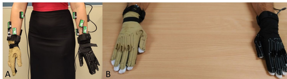
Fig. 1 (A) Participant equipped with Biometrics sEMG electrodes (LE230) and CyberGlove data gloves. (B) Hand reference posture for kinematics recording.
