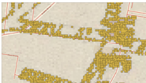
Fig. 3 A vector layer for a road segment that has not been reclassified. Yellow polygons demonstrate the discrete and non-homogenized pixels emerged from vectorization.
