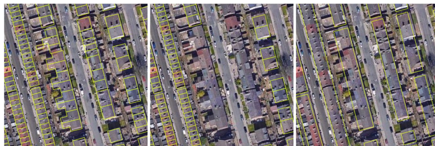
Fig. 2 Building outline polygons of three available datasets visualized on aerial images. UKBuildings 26 (left), OSM 27 (center), and OS OpenMap 28 (right) on Google Maps aerial image.
