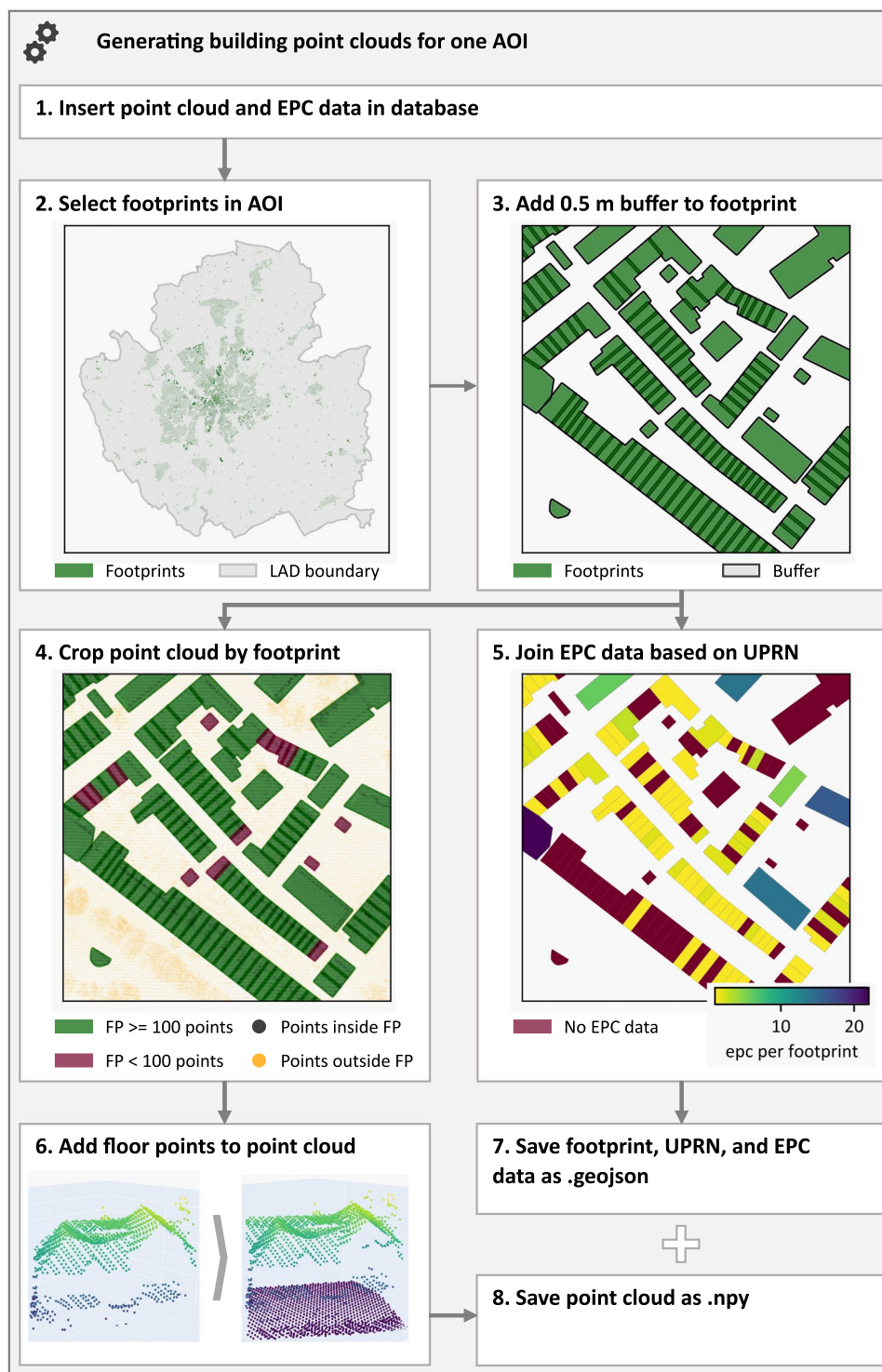
Fig. 4 Overview and visualization of the program's steps for generating building point clouds and their energy characteristics for one AOI.
