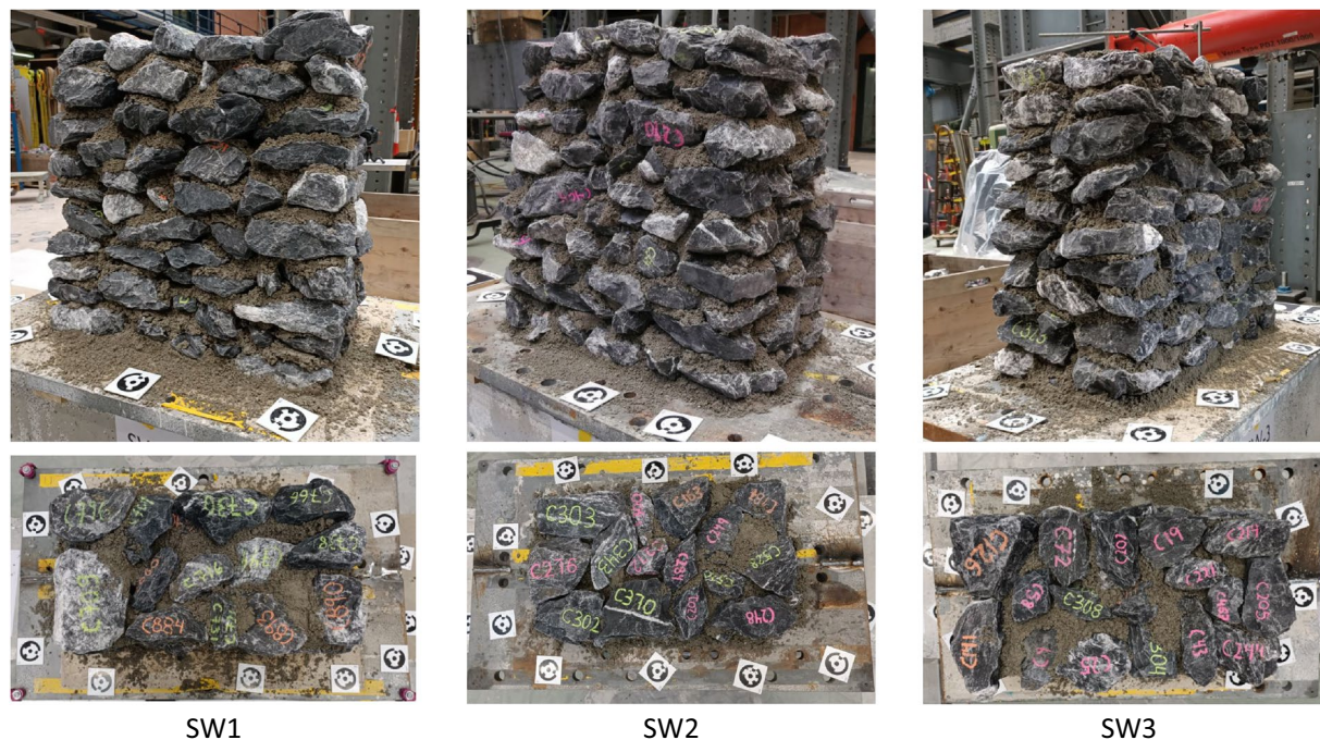
Fig. 1 The three rubble stone masonry walls (top) and representative sections with the distribution of the stones through the thickness (bottom) used in this study. From left to right, the walls are labeled SW1, SW2, SW3. For scale purposes, consider that the side of the square markers is 80 mm and the diameter of the black circles 65 mm.
