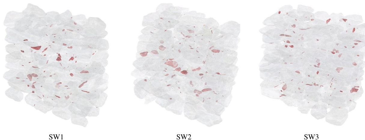
Fig. 12 Visualisation of the colliding volumes (in red) within each wall at the first application of the collision analysis algorithm during the digital reconstruction process. Stone meshes are shown in transparent.
