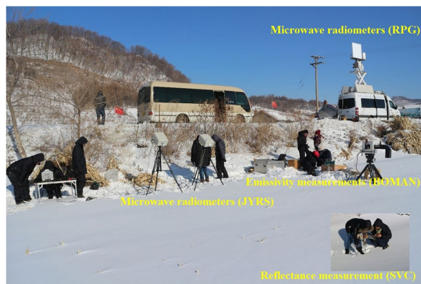
Fig. 3 The full-band spectra (i.e., reflectance, thermal emissivity, microwave emission) measurements over a snow surface in Jiaohe of Jilin province.
