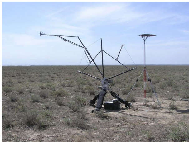
Fig. 4 A typical multi-angular reflectance spectra measurement with a portable multi-angle observation device.
