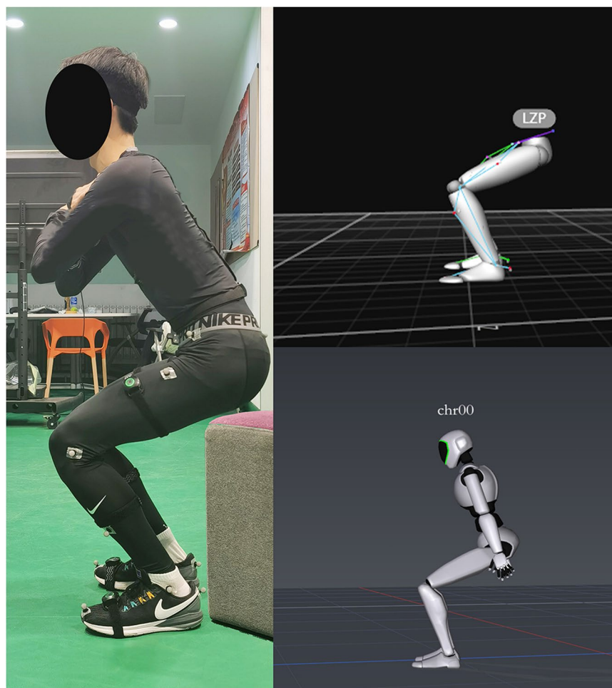
Fig. 6 Lower limb task, and comparison chart of OptiTrack and PNS.
