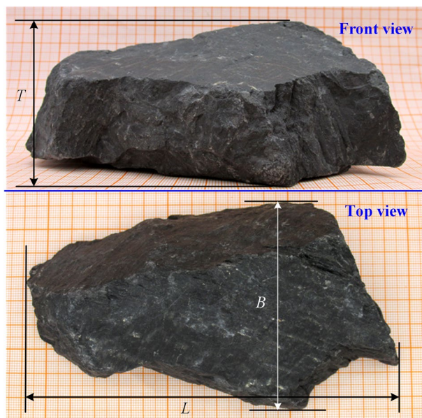
Fig. 6 Triaxial diameter measurement method.
