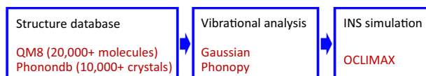
Fig. 1 Workflow used to produce the INS spectra database. The QM8 database was used for organic molecules, and the Phonondb was used for inorganic crystals. The vibrational analysis was performed using Gaussian 09 and Phonopy codes, and the resulting INS simulation was produced using OCLIMAX software.
