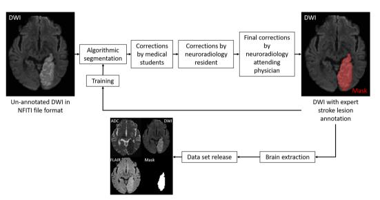
Fig. 2 Workflow graphic of the hybrid human-algorithm stroke lesion segmentation applied in this dataset.
