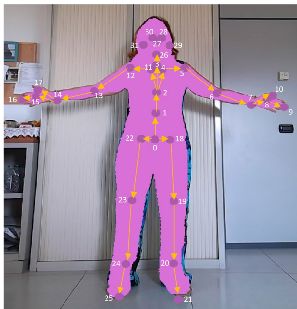
Fig. 6 Joint locations and connections relative to the human skeleton extracted using the Microsoft Azure Kinect Body Tracking SDK v1.1.2 19 . The skeleton includes 32 joints, numbered from 0 to 31, with the joint hierarchy flowing from the center of the body to the extremities.
