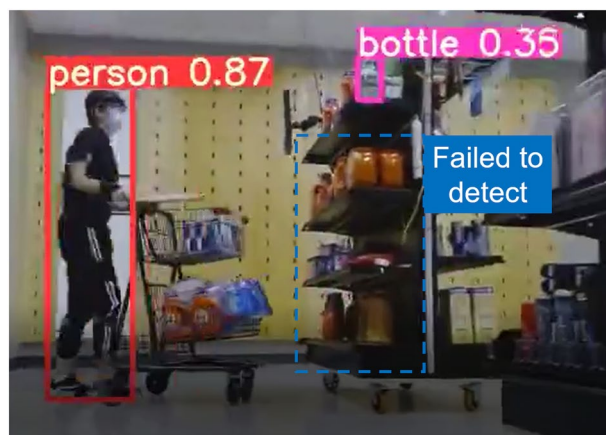
Fig. 5 A demonstration figure of the video frame annotated by YOLO V5. The participant consented for the publication to utilize their likenesses.
