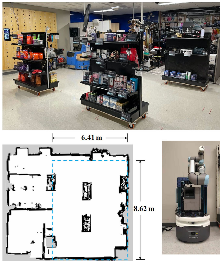
Fig. 1 Top: a picture of the future-oriented WRT research facility. Bottom Left: 2D costmap of the facility and dimensions of the experiment area. Bottom Right: a picture of the customized mobile robot platform used in the experiment.
