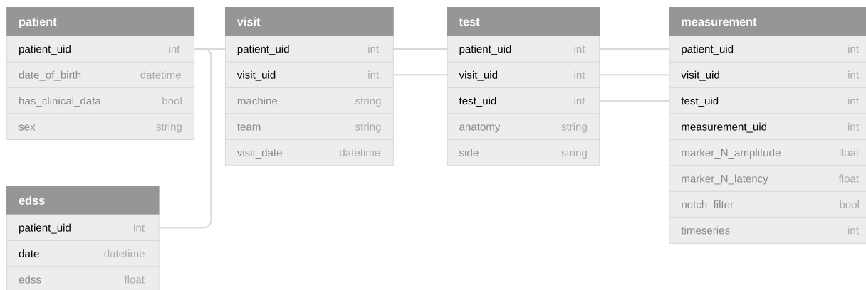
Fig. 5 A schematic overview of the tables in the dataset. Per table, all the bold fields combine to make a unique identifier for a record in that table (composite key). Section Data Records contains descriptions of each of the fields.
