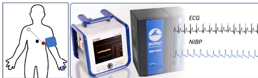
Fig. 1 Cardiovascular recordings using system 1 - the Task Force Monitor (CNSystems), or system 2 - the CNAP 500 (CNSystems) combined with an MP150 acquisition unit (BIOPAC Systems Inc.). Top left: In System 1, four electrodes have been attached at the right arm (red), the left arm (yellow), the left abdomen (green), and the right abdomen (black). Two ECG channels have been recorded between the electrodes red and yellow (lead I), and between red and green (lead II). Pressure cuffs have been attached around the left arm as well as left middle and index finger. Top right: Two ECG leads were sampled synchronously at 1000 Hz and the continuous blood pressure signal at 100 Hz. Bottom left: In System 2, three electrodes have been attached below the centre of the right clavicle (white), at the left lower thorax (7th intracoastal space at midclavicular line) (red), and at the sternum (black). One ECG channel has been recorded between the electrodes red and white (lead II). Pressure cuffs were attached around the left arm as well as left middle and index finger. Bottom right: The ECG was sampled synchronously at 1000 Hz and the continuous blood pressure signal at 100 Hz. Pictures from www.cnsystems.com and www.biopac.com adapted with permission.
