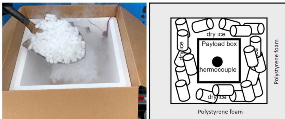
Fig. 8 package with loaded dry ice and payload box insider (Test 2).
