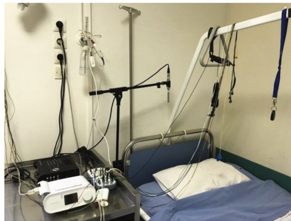
Fig. 1 Contact and ambient microphones installed in the sleep study room, along with the multitrack recorder.
