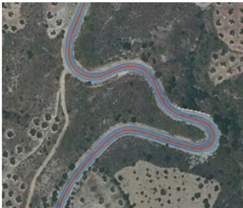
Fig. 6 The results of the survey of the two white roadside lines (in blue) and the mean axis or control axis (in red).
