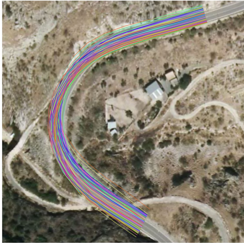
Fig. 1 Example illustrating multitracess. Each coloured line represents a different trace. Basemap: Orthophoto from Instituto Geográfico Nacional.
