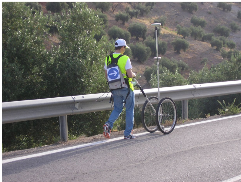
Fig. 5 Precise GNSS survey using the Leica 1200 system.
