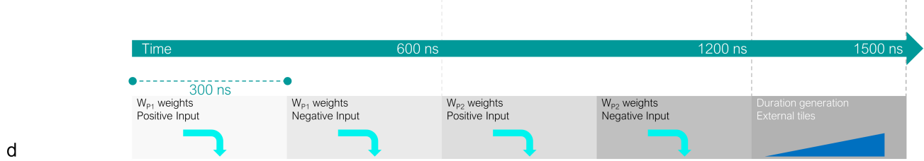
Extended Data Fig. 7 | MLPerfRNNT Decoder mapping and signal routing on chip. Instead of processing Embedding Emb and Dec-LSTM0 W_x layers separately, we first compress in one single matrix the product Emb * W_x . At this point, the first Dec-LSTM0 shows Emb * W_x matrix with a (28*1280) size, contrasting with the (320*1280) W_h size to sum directly in analog. To balance signal magnitude, nine copies of Emb * (W_x/9) are programmed, achieving
