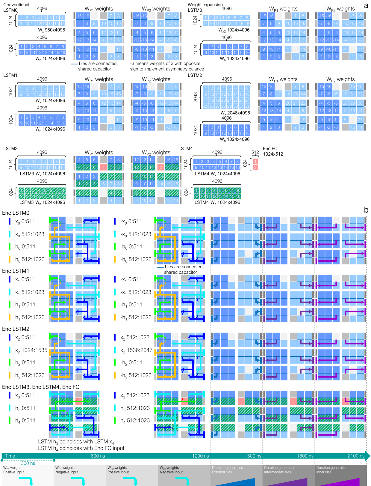
Extended Data Fig. 5 | MLPPerfRNT Encoder mapping and signal routing on chip. (a) RNN Encoder LSTMs weights are represented by two large matrices, W_x which multiplies the LSTM input, x , and W_h which multiplies the LSTM recurrent signal, h . Depending on the sizes of x and h , a variable number of tiles is required. Both conventional and weight expansion mappings are shown for Enc-LSTM0. In addition, Enc-LSTM0, Enc-LSTM1 and the W_h of Enc-LSTM2 implement Asymmetry Balance. Tiles connected with a dark blue line have shared capacitors, enabling 2048-wide analog MAC. In Enc-LSTM0, Enc-LSTM1
