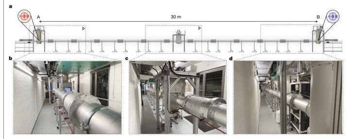
**Fig. 3** | **Cryogenic microwave quantum link. a**, Computer-aided design (CAD) model. **b**-**d**, Photographs of the 30-m-long cryogenic set-up. Dilution refrigerators at each end host the quantum devices that are connected through a waveguide cooled to below 50 mK over the full distance. A central pulse tube
