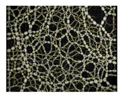
From cell monolayers to modern architecture, two-dimensional disordered structures confer remarkable robustness and flexibility. But mitigating the effects of failure in these materials is a task complicated by their heterogeneity. Now, Estelle Berthier and colleagues have taken inspiration from network science to forecast failure locations by comparing the importance of connections within the disordered lattice.
