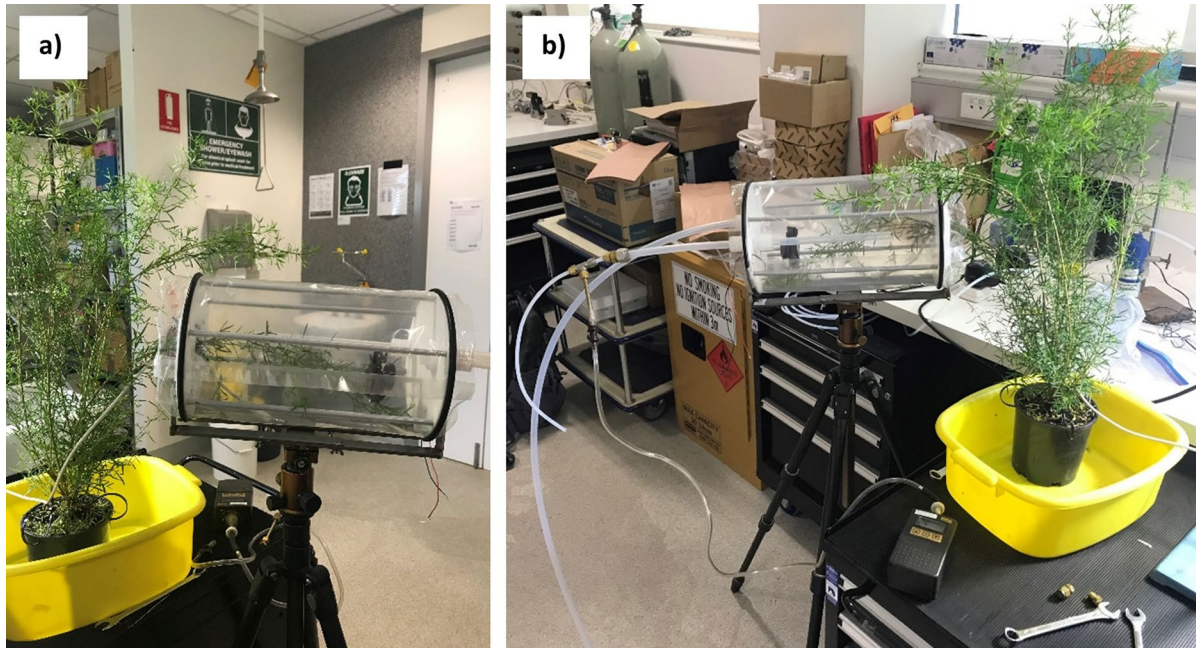
Extended Data Fig. 8 | Sampling B. pinnata VOC emission rate. a) Here, a single branch of a B. pinnata was placed inside a custom-built branch enclosure chamber. b) An air pump, connected to the chamber via plastic tubing draws air out of the chamber, and through a sorbent tube where the VOCs emitted by the
