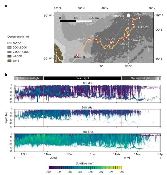
**Fig. 1**|Acoustic backscatter during the drift of the autonomous sea ice observatory. a, Map showing monthly drift positions. Bathymetry: International Bathymetric Chart of the Arctic Ocean (IBCAO) v.4.0 (ref. 55). b, Time series plot of mean volume backscattering strength ( $S_v$ ) at 125, 200 and 455 kHz for the
