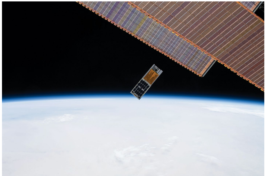
Fig. 1 | HaloSat just after deployment from the ISS. HaloSat and RainCube, a CubeSat from the Jet Propulsion Laboratory, are seen in the centre. RainCube is in front of the Earth's limb, while HaloSat has a gold thermal shield. The two CubeSats have identical dimensions while stowed and are touching when deployed, but not physically attached. They separated a few minutes after this photograph was taken and are now tens of kilometres apart. Parts of the ISS's solar array are visible in the upper right. Credit: NASA
