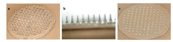
Fig. 1 Fabrication of dissolving microneedle patch (dMNP). First-generation dMNP was composed of 112 microneedles (a), each MN measuring 700  $\mu$ m in length, occupying an ~0.8 cm<sup>2</sup> area mounted on an adhesive backing (b). Microneedles were dissolved after insertion into the skin of a rat (c).
