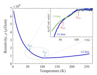
Fig. 3 Resistivity vs temperature at near-ambient pressure. The temperature of the resistivity minimum,  $T_{\min}$ , is marked with an arrow. The inset shows the result of differentiating the data with respect to temperature, which reveals a subtle kink or shoulder around 60 K, Tkink.
