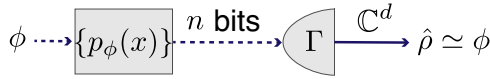
Fig. 2 Probabilistic encoding of pure state \phi on a d -dimensional system using n -bit strings and a decoder \Gamma that generates an approximated state \hat{\rho} . State \phi is probabilistically encoded in label x in a finite set X in accordance with probability distribution p_\phi: X \rightarrow [0, 1] . As a special case of probabilistic encoding, we also consider deterministic encoding that utilizes probability distribution p_\phi: X \rightarrow \{0, 1\} . Note that the length of classical bit strings to represent x \in X is given by n = \lceil \log_2 |X| \rceil .
