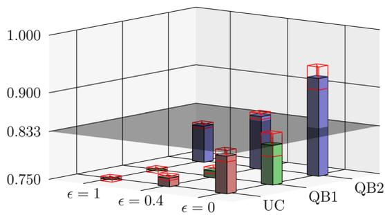
**Fig. 6** Experimentally measured average cloning fidelity  $\bar{F}_i$  for quantum banknotes 1 and 2 (QB1 and QB2), and optimal universal cloning (UC). The red frames show the error bars of the measured probabilities. The verification threshold (gray surface) is set at 0.833, which is the fidelity of the optimal universal cloning process, i.e., the process that ignores any information about  $g$
