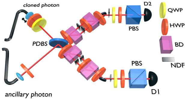
**Fig. 3** Experimental setup for cloning quantum banknotes. Components are labeled as follows: HWP is half-wave plate, QWP is quarter wave-plate, PDBS is polarization dependent-beam splitter, PBS is polarizing beam splitter, BD is beam divider, NDF is neutral density filter, and D is single photon detector. A successful cloning and verification of a qubit from a given sequence is registered as a simultaneous detection event at the two detectors
