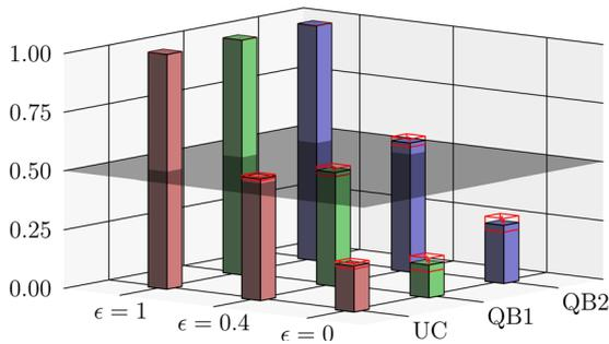
**Fig. 5** Success probabilities of the cloning processes for quantum banknotes 1 and 2 (QB1 and QB2), and optimal universal cloning (UC). The red frames show the error bars of the measured probabilities. The gray surface shows the minimum cloning efficiency needed to output on average more cloned photons than the input photons
