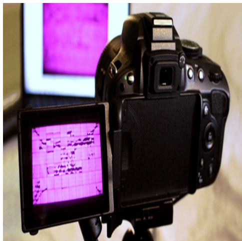
Fig. 6 EL imaging setup used to test the PV module. The EL camera is brought by Brightspot Automation, USA-based company.
