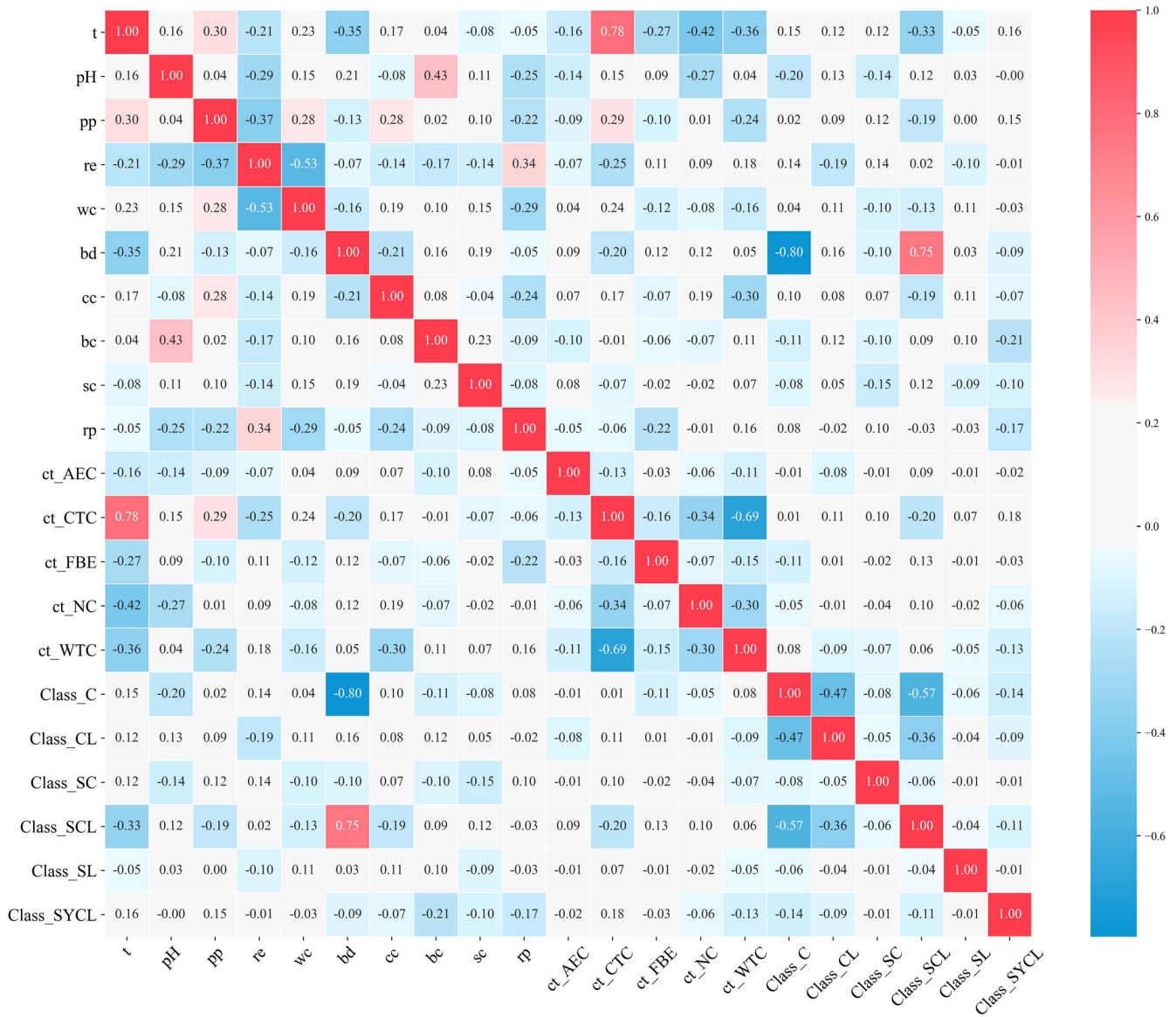
Fig. 4 Matrix of the Spearman correlation coefficients between the different features. Strongly correlated (>0.7) features indicate the presence of redundant variables, which guide the screening of features.
