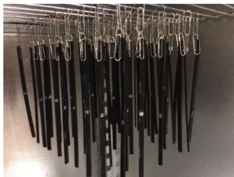
Fig. 10 The specimens in the aging oven. Vulcanizate strips are hung dispersedly in the temperature-controlled air-aging oven to ensure uniformly aging.
