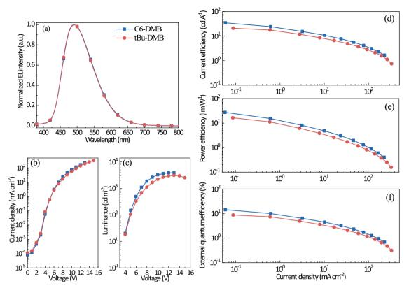
Fig. 6 Device performance of non-doped devices. a EL spectra; b current density to voltage curves; c luminance to voltage curves; d current efficiency to current density curves; f EQE to current density curves of non-doped devices.
