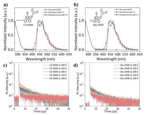
Fig. 4 Photophysical properties. UV–vis absorption spectra, fluorescence, and phosphorescence spectra at 77 K of (a) C6-DMB and (b) tBu-DMB. Temperature-dependent transient PL decay characteristics of (c) C6-DMB and (d) tBu-DMB in doped (30 wt%) mCP films.
