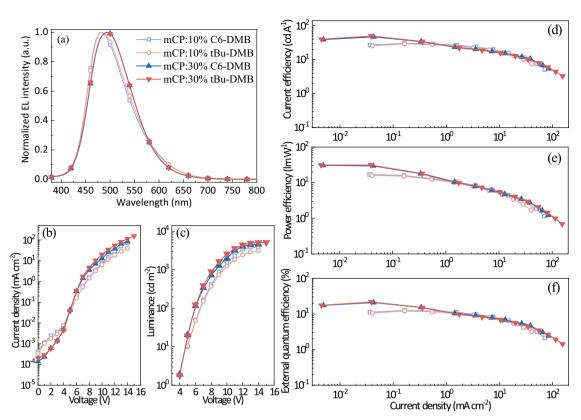
Fig. 5 Device performance of doped devices. a EL spectra; b current density to voltage curves; c luminance to voltage curves; d current efficiency to current density curves; f EQE to current density curves of doped devices.
