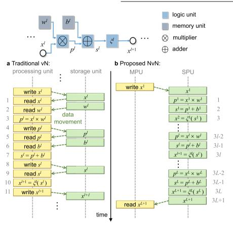
**Fig. 9** Schematic comparison of calculation step between vN and NvN architecture. Equation (7) is used as an example to indicate the difference between traditional vN architecture (**a**) and proposed NvN architecture (**b**) based on the processing-in-memory (PIM) technology. Here  $x'_i$ ,  $w'_i$ ,  $b'_i$ , and  $\xi'_i$  are input, weight, bias, and nonlinear activation function of the  $I^{\text{th}}$  layer, respectively;  $p' = x' \times w'_i$ ; s' = b' + p'.
